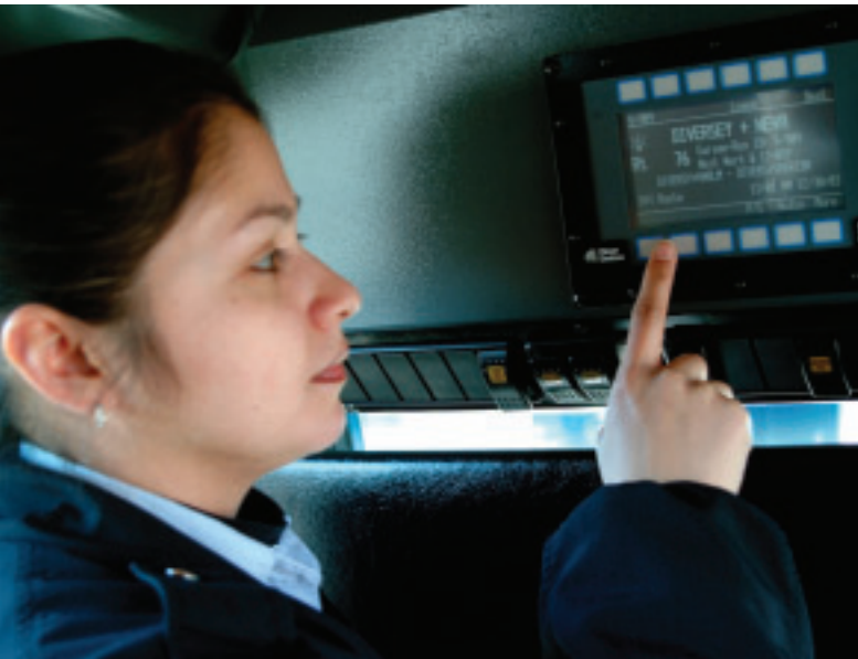
A CTA bus operator programs the automated bus announcement system that provides audible announcements on CTA buses and electronic signs that display the upcoming stop.
