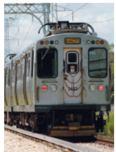
The CTA replaced the overhead catenary lines used to power the Yellow Line with contact rail, or third rail, like that used everywhere else on the CTA system.
