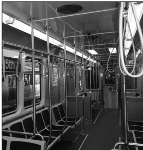
The 5000 series rail cars feature aisle-facing seating designed to allow more room for customers and items they bring onboard, as well as more space for standing customers.
