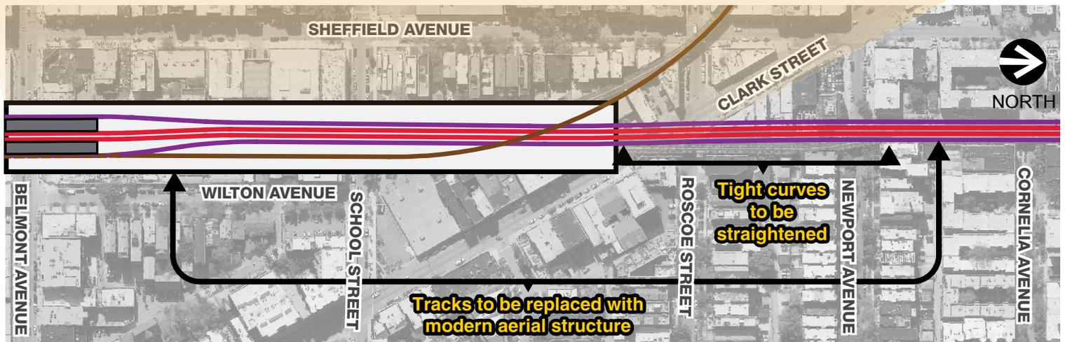
Schematic of the Red-Purple Bypass Project Build Alternative
