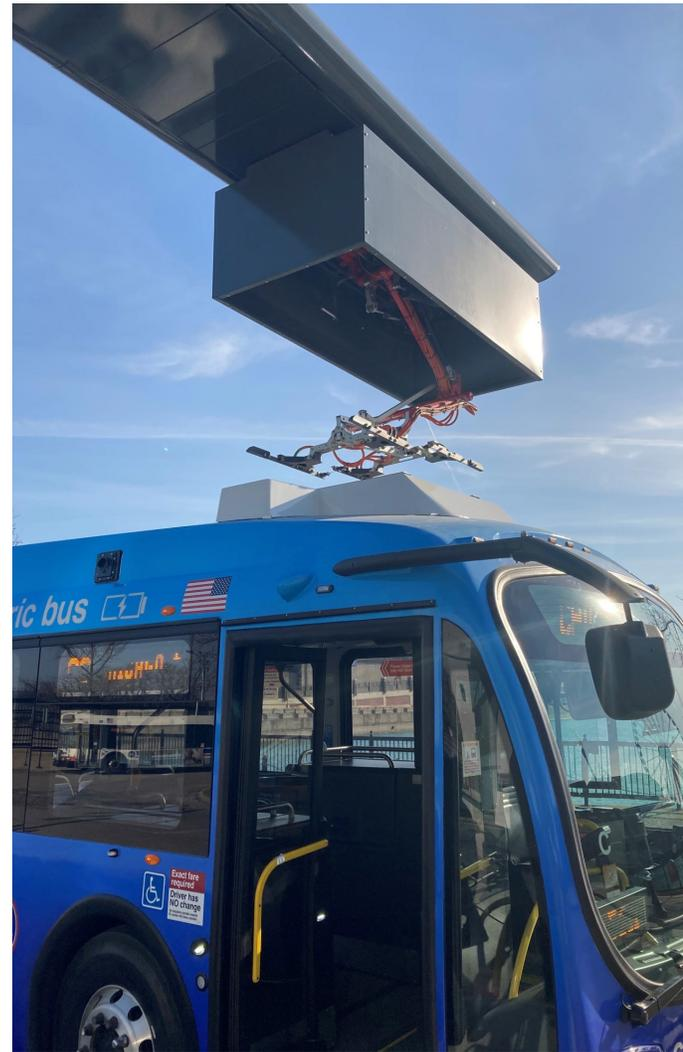
Figure 4 - Photo of pantograph charger at Navy Pier
